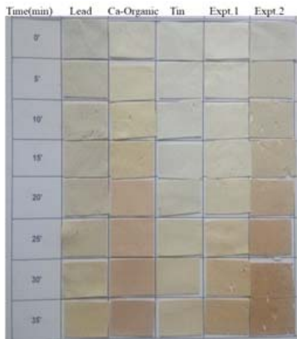
Fig 5. Oven Stability test for stabilizers. Color changes of PVC strips at 190°C.
