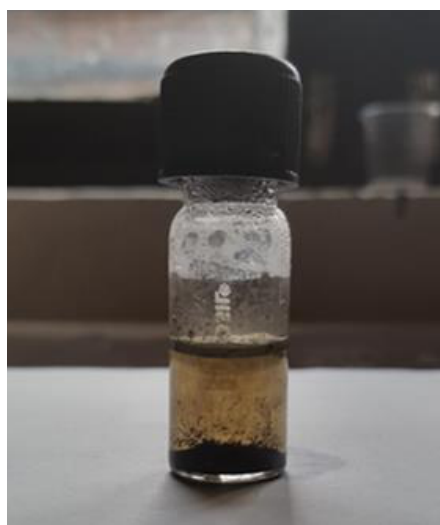
Fig. 3. Photographs showing different stages of stable precipitate: (a) agglomerated MNPs settling down in the glass vial, and (b) TMAOH-coated MNPs which stayed stable for months
