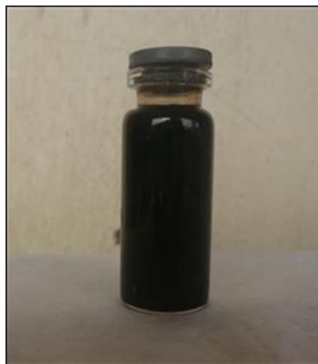
Fig. 3. Photographs showing different stages of stable precipitate: (a) agglomerated MNPs settling down in the glass vial, and (b) TMAOH-coated MNPs which stayed stable for months
